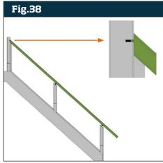
To cut handrail to correct length, measure approx. 25mm away from connector 1 at bottom of handrail, mark and cut rail square (Fig.39).
