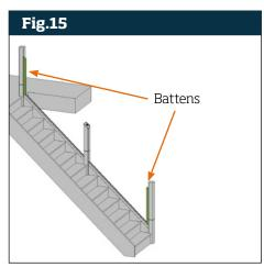
Offer handrail assembly between top and bottom newels and onto tops of battens with threaded fasteners located to side of newel faces on stair side. Mark fastener location on bottom and top newels (Fig.16).
